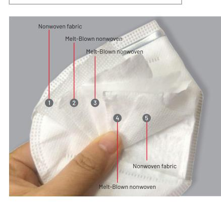
Efficient personal protection equipment to protect the respiratory tract from fumes, dusts and aerosols. With a classic cup shape which covers the mouth and nose and also allows it to be folded.
