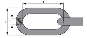
Grade 80 chain is designed to ensure lifting and pulling operations, being the main element of steel slings which, in combination with different accessories and a correct calculation of the maximum loads, guarantees highly safe operations.
