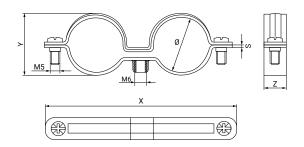
This clamp is usually fixed to ceilings and enables to pass two parallel pipes of any desired diameter. It is fixed to the wall by means of a lag screw and a plug where the double clamp is screwed on.
