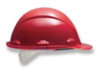
This high-density polyethylene protective helmet is suitable for work near active electrical conductors and where there is a risk of being hit by falling objects. It has an impact resistance of  $-10^\circ$  C/50° C and an electrical insulation of up to 400 V ac. In addition, it has an anti-allergic sweatband and pin-hole adjustment.
