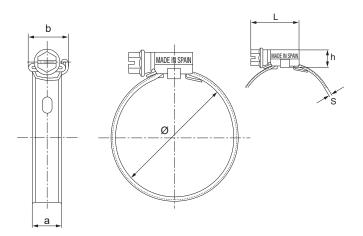
With the aim of minimising costs on the assembly line, particularly in the automotive sector, Mikalor has developed an ASFA clamp incorporating a pre-positioning notch in the band. This clamp works at the same tightening torque and guarantees the same performance as the standard range.
