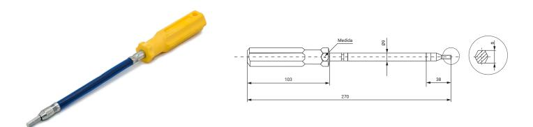
Screwdriver with flexible shank and hexagon socket for tightening the screw of the clamps even if the screwdriver is not completely aligned with the screw. Its handle is ergonomic and made of a suitable material for a perfect grip, so it does not slip during use.
