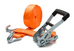
This ratchet set consists of a tensioning device with a sewn band with a closed hook end and another band section with a closed hook end.
