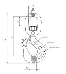
Its convenient design, careful forging and controlled precision of the heat treatment result in the maximum working load without excessive hook weight and size. A DIN 1481 pin set in the centre of the nut and in the threaded part of the hook provides a perfect connection that prevents loosening and guarantees maximum functional safety.
