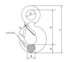
The quality of the latch-activating spring makes it fast to operate without altering the safety level required by the process of lifting or moving loads. Each hook is marked with its working load in tonnes and with the material-identifying symbol: (C) for carbon steel hooks and (A) for alloy steel hooks, guaranteeing the correct choice.
