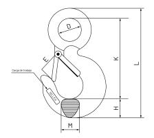
The quality of the latch-activating spring makes it fast to operate without altering the safety level required by the process of lifting or moving loads. Each hook is marked with its working load in tonnes and with the material-identifying symbol: (C) for carbon steel hooks and (A) for alloy steel hooks, guaranteeing the correct choice.
