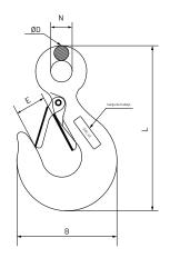
The quality of the latch-activating spring makes it fast to operate without altering the safety level required by the process of lifting or moving loads. Each hook is marked with its working load in tonnes and with the material-identifying symbol: (C) for carbon steel hooks and (A) for alloy steel hooks, guaranteeing the correct choice.
