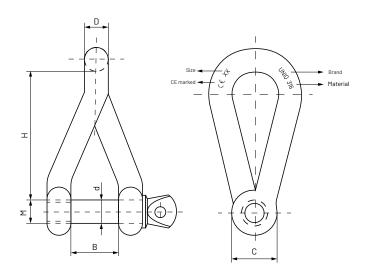
The  $90^{\circ}$  rotation of the shackle bow is really useful when the stress is perpendicular to the shackle shaft.
