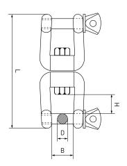
It is used just like a standard shackle, removing the bolt allows for an easy assembly inside the structure of the element to be lifted or fastened. They differ from the standard shackle in that, if there are directional or opposite rotating movements, they prevent chains, wires or ropes from twisting as these are 2 independent rotating parts.
