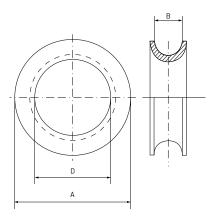
The wire rope thimble is an essential element to protect the wire from any kind of friction.
