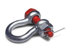
Each shackle is marked with its size and its working load in tonnes, guaranteeing the correct choice and, therefore, increasing safety. The widening of the bow makes it easier to accommodate the sling or hook of choice, and can improve mobility if necessary. The hex-head screw with nut and pin, which acts as a bolt increases the required safety level.
