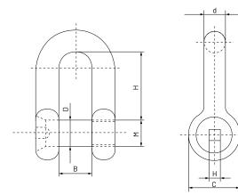
The high-resistance steel component of its structure ensures that great working loads can be lifted with a smaller shackle. Besides, its socket head ensures greater safety when lifting loads.
