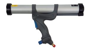
The lightweight pneumatic dispensing tool was designed for industrial applications. It works at 1,5kN and has a working pressure of 6.8 bars. It has a direct action mechanism and is very quiet (less than 70dB). This tool is very compact and incorporates an integrated regulator. Suitable for the application of both high and low viscosity anchors.
