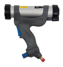
The lightweight pneumatic dispensing tool was designed for industrial applications. It works at 1,5kN and has a working pressure of 6.8 bars. It has a direct action mechanism and is very quiet (less than 70dB). This tool is very compact and allows for the fast and effortless application of both high and low viscosity anchors.
