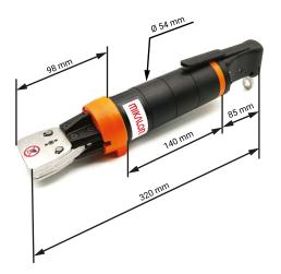
The pneumatic tool is ideal for the full range of ear clamps, including inner-ring ear clips, clip clamps and OEM ear clips. It also has a high capacity for series assembly. Its working pressure is 6 bar.
