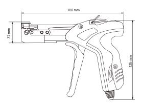
Cable Tie Gun for the assembly of stainless steel cable ties. It incorporates a function which regulates tension in the band and cuts off the band end automatically after tightening.
