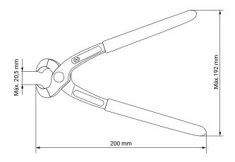
These pincers can be used to fasten all types of ear clip. The front-closing model is the most popular type and is used in most ear-clip assemblies. It is also known as the "Russian" model.
