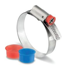
The Safety Collar is an ideal solution which prevents the screwdriver from slipping out of the slot in the screw while tightening. It is easy to assemble and extremely useful. The slot is easily accessible while the collar helps to hold the screwdriver in place. Available in two colours, red and blue, which help to identify the material quality of the clamp.
