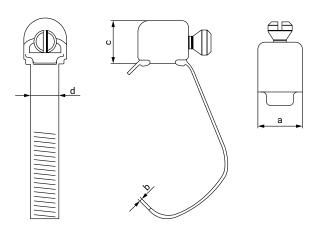
The reduced dimensions of the housing of this clip make it the ideal choice for applications where space is at a premium. This clip is delivered open, making it suitable for use in difficult applications with little space to manoeuvre.
