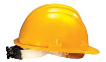
This high-density polyethylene protective helmet is suitable for work near active electrical conductors and where there is a risk of being hit by falling objects. It has an impact resistance of  $-20^{\circ}$  C/ $50^{\circ}$  C and an electrical insulation of up to 400 V ac. In addition, it has an anti-allergic sweatband and a wheel fastener.
