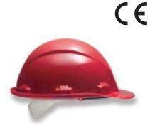
This high-density polyethylene protective helmet is suitable for work near active electrical conductors and where there is a risk of being hit by falling objects. It has an impact resistance of  $-10^{\circ}$  C/50° C and an electrical insulation of up to 400 V ac. In addition, it has an anti-allergic sweatband and pin-hole adjustment.
