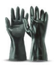
Neoprene gloves are made of polychloroprene and latex without liner in a fabric form and have a long cuff and inner cotton flocking. The length of the glove is 31 cm, the thickness is 0.70 mm and the cut is straight. They have high abrasion resistance and excellent flexibility, which is why they are especially suitable for the chemical and petrochemical industry, automotive, heavy maintenance work and industrial cleaning.
