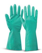
These gloves are made of non-slip green acrylonitrile, without liner, have a long cuff and an internal cotton flocking. The length of the glove is 33 cm, the thickness is 0.38 mm and the cut is straight. They have very good resistance to abrasion and solvents, which is why they are especially suitable for handling solvents, paint and alcohols. They are recommended for the paint and varnish industry, chemical and petrochemical industry, graphic and printing industries.
