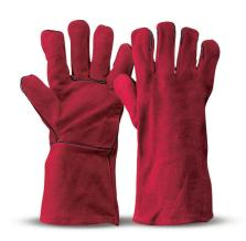
These gloves feature an extra-quality calfskin palm, KEVLAR® fibre reinforcement seams on the palm with flame protection, fully lined inner fabric for increased heat protection and a 15 cm leather cuff. They are especially indicated for works with heat risks, risks of handling hot objects and welding.
