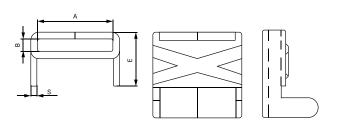
This stainless steel buckle is specific for the lightweight SS endless band, but can also be used for the heavy-duty series. Prevents the band from coming loose after it has been placed. Pressure is exerted on the band when the buckle is tapped, preventing it from coming loose.
