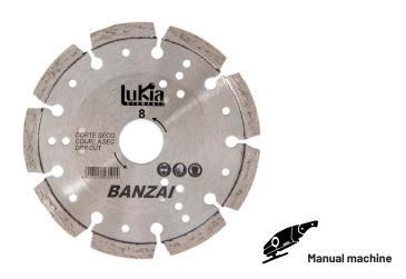
This blade is laser-welded for extra resistance for cutting materials with a high iron content and even with rods in their composition. It has a segmented blade, which stands out for offering great power, higher cutting speed and very good air cooling.
