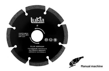
This blade is perfect for dry cutting and suitable for cutting building materials that are excessively hard or abrasive (asphalt, fresh concrete, old concrete, abrasive terracotta, grinding stone, etc.). This blade is made of a special abrasive material to resist wear. It has a segmented blade, which stands out for offering great power, higher cutting speed and very good air cooling.
