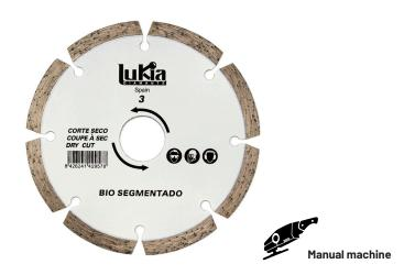
This blade is perfect for dry cutting and suitable for cutting building materials that are not excessively hard or abrasive (construction brick, soft stone, masonry, cement tiles, ceramic tiles, concrete, etc.). It has a segmented blade, which stands out for offering great power, higher cutting speed and very good air cooling.
