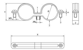
This clamp is usually fixed to ceilings and enables to pass two parallel pipes of any desired diameter. It is fixed to the wall by means of a lag screw and a plug where the double clamp is screwed on.
