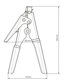
Fastening tool for nylon cable ties from 3,6 mm to 10,6 mm wide and from 1,2 mm to 2,3 mm thick. When maximum tension is reached, the cutting
