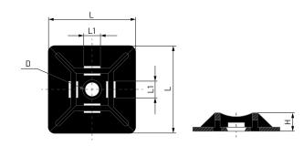
The self-adhesive cable tie mounts are available in 2 colours, black and white, and different sizes for different nylon cable tie widths. They are perfect for quick fastenings on plain walls, held in place by a cable tie without the need to drill holes. The side of the self-adhesive cable tie mount opposite to the surface that adheres to the wall has 4 cavities on each of its sides to pass through the nylon cable tie in order to fasten the desired element
