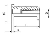
Rivet nuts are used both to join several metal sheets and assemble a threaded element.
