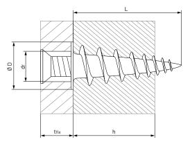
The plasterboard nylon plug is especially suitable for cardboard sheets, plaster and plasterboard sheets. When introduced into hollow spaces, it expands and provides a perfect grip on this type of surface.
