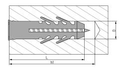
It works just as the conventional nylon plug. The difference is that it has two wings at the end of the plug, with a hole in each wing to pass through a nylon cable tie and secure it. This enables fixing any element on solid materials. Once the plug has been inserted into the hole, the wings are visible so that the desired nylon cable tie can be passed through.
