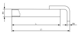
A 47 mm diameter tube with an 18 mm extension at its end, which is also made of steel, fixes the scaffold to the façade. The extension at one end is fixed to the scaffold by means of a clamp and, at the other end, the L-shaped extension is inserted into the 24 mm diameter ring, thus fixing the scaffold to the façade.
