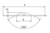
This special fastening washer together with the rib that we will place in his central hole, is used to fix isolation panels of fiberglass.
