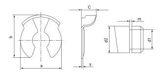
The CL shaft clip is particularly useful for use with small diameter shafts as it can handle quite considerable axial forces.
