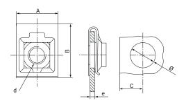
The TCL Special Cage nut is a fastener composed of two flaps in clip form. A multi-thread square nut is set into the centre of the upper flap which when given the correct torque can give maximum fastening and assembly strength.
