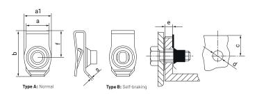
The TRT chimney nut is a fastener composed of two flaps in clip form. The design of this nut means that a double elastic force is exerted when tightened. In the middle of the upper flap there is a hollow cylinder or "chimney" with multiple threads which when given the correct torque guarantees maximum fastening and assembly strength. The lower flap incorporates a third flap which is set in the opposite direction to the outer flaps in order to ensure optimum grip on the panel.
