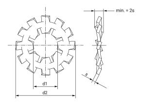
This washer is used in panel assembly using holes and groves which are much bigger than the diameter of the screw or bolt, in order to achieve evenly distributed pressure over the entire area of contact.
