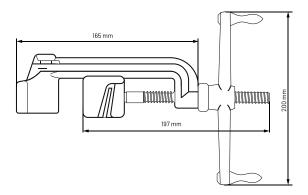
This tool is designed for both the lightweight and heavy-duty SS endless band to achieve the appropriate tension and make a clean final cut.
