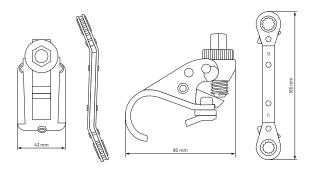
This tool is used together with the turnbuckle to make the final cut and avoid parts protruding beyond the fixed diameter, thus avoiding damage due to scratches or tears.
