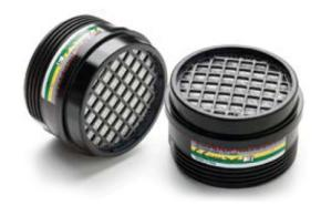
The FMABEKP mask filter consists of a high density polyethylene (HDPE) spin-on cartridge with activated carbon and non-woven polypropylene (PP) inside. Each filter, designed to optimize the field of vision, carries a color-coded label in brown, grey, yellow, green and white that identifies the type of protection it can offer. Resistance to breathing:
